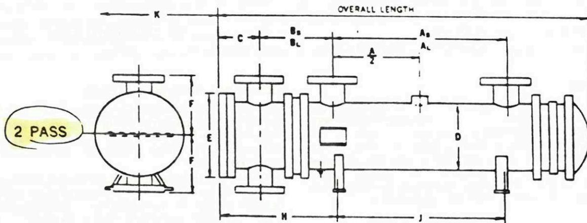
**NOTE:** Flanges for field connections drilled and faced per 150# ANSI standards.
